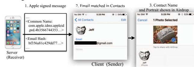
Figure 4: The process of checking contacts in Airdrop
